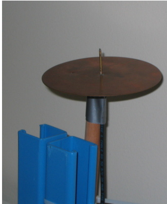
Figure 4.1 Picture of transmitter antenna, a custom-built 2.45 GHz quarter-wavelength monopole with circular ground plane.
