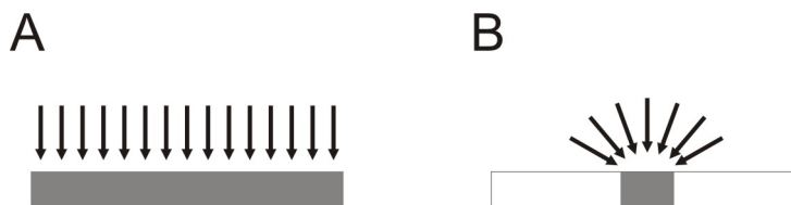
Figure 2.2. Schematic representation of planar (A) and hemispherical (B) diffusion.
