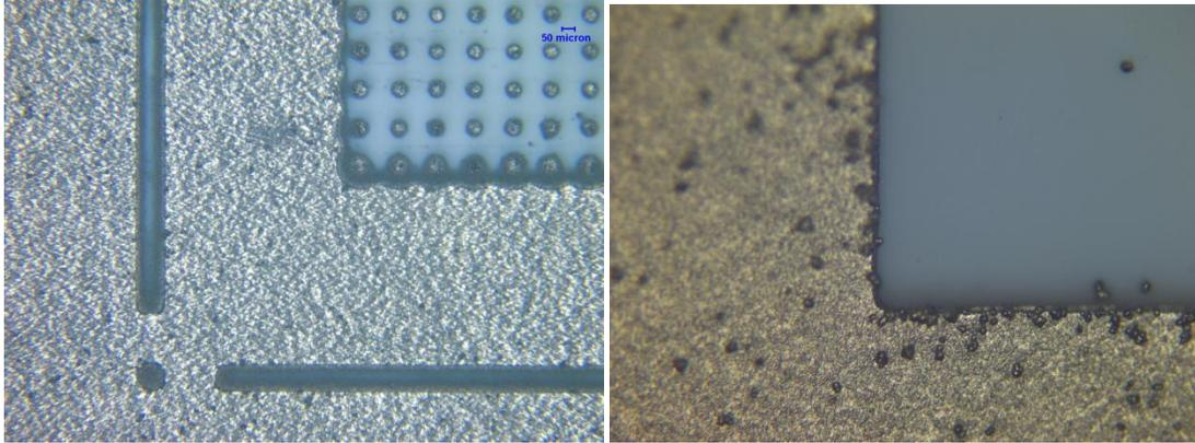
Figure 16. Optical photomicrographs of a patterned LCP second generation sample, showing the layout of multiple feedthrough pads (left), and of an unpatterned LCP second generation sample (right).
