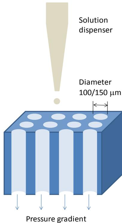
Figure 3: Schematic for sol-gel infiltration process
