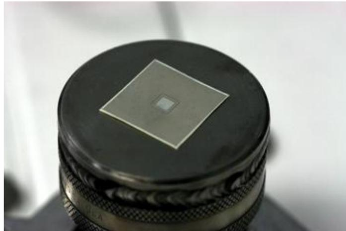
Figure 17. Second generation bare LCP sample mounted to the vacuum chuck atop the He leak detector measurement flange with Dow Corning® vacuum grease to form a vacuum seal.
