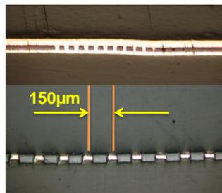
Fig 13: Cross-section of metalized LCP vias at 150µm pitch
