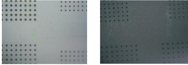
(a) Top view optical image of laser drilled LCP      (b) Optical image after electroless Pd deposition
