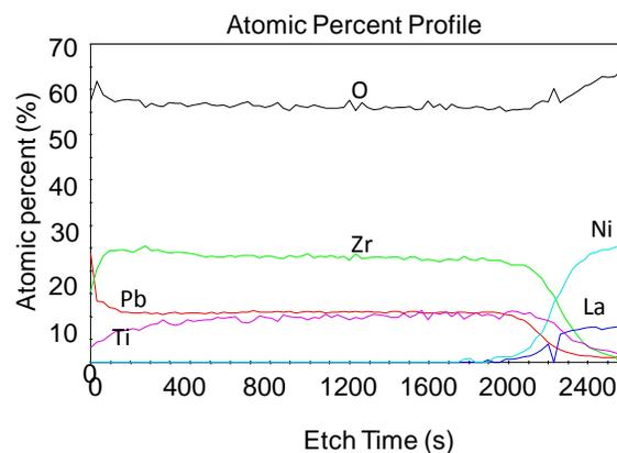
Figure 7: XPS compositional depth profile of the planar films
