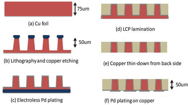
Figure 14: Process flow schematic for 'vialess' process
