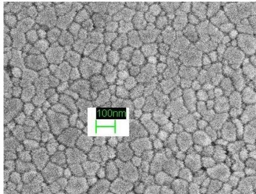
(a) Top view of the sol-gel PZT thin film
