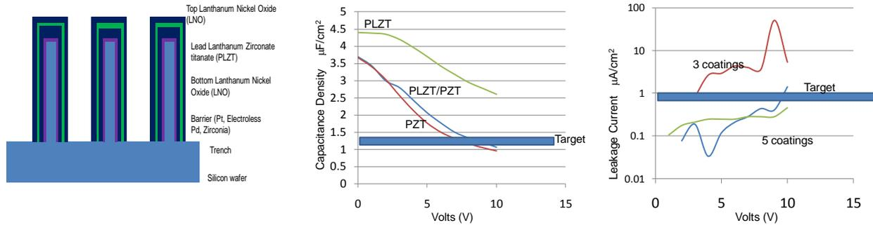
Figure 1: Key capacitance density and leakage current targets from year 1.
