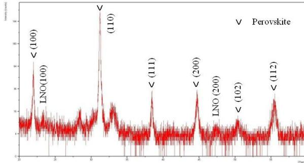
Figure 5: XRD result for PZT/LNO/SiO<sub>2</sub>/Si planar device.
