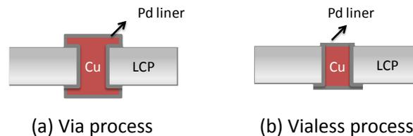
Figure 10: Schematic cross-section of vertical feed-through in LCP
