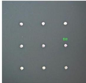
Figure 12: Selective palladium deposition on LCP using photoresist lift-off method showing 75µm diameter features
