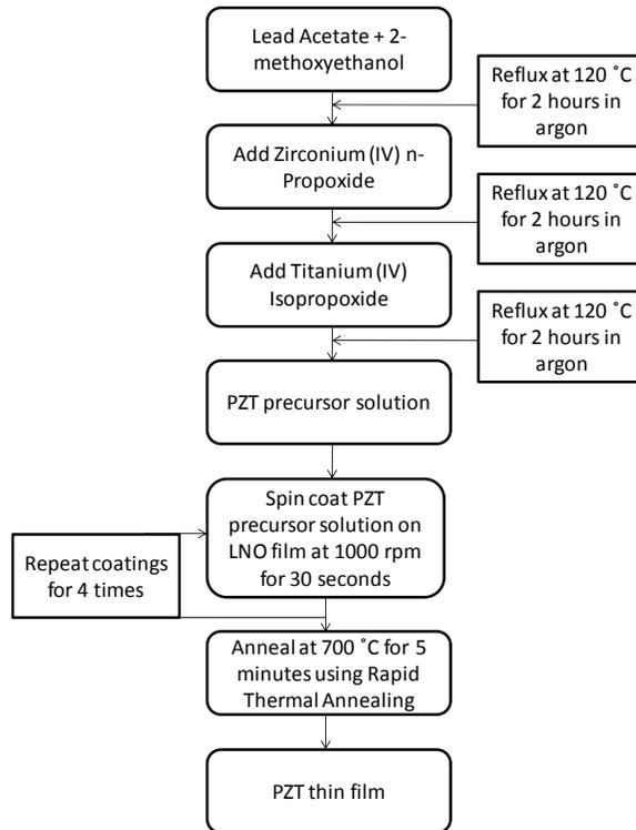
Figure 2: Flow chart for the PZT sol-gel process
