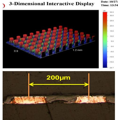
Fig 15: Image of copper pillar array, cross-section of LCP with Cu feedthrough
