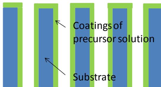
Figure 4: 3D structure after sol-gel vacuum-infiltration
