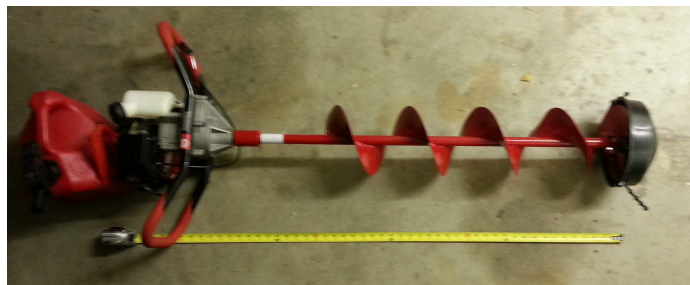
Figure 27: Auger used to drill ice deployment hole and as a feature for the sonar and video sensors
