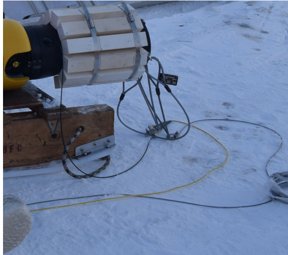
Figure 20: Rear thruster module with the optical fiber tether (yellow) and the steel strength support cable (gray)
