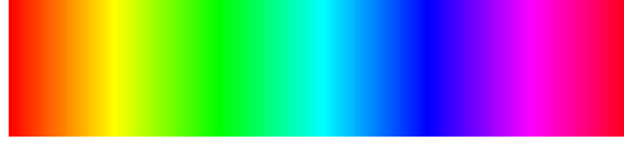
Figure 63: Hue spectrum which typically varies from 0 to 359, but here is divided by two to fit into an 8-bit representation, and so varies from 0 to 179.
