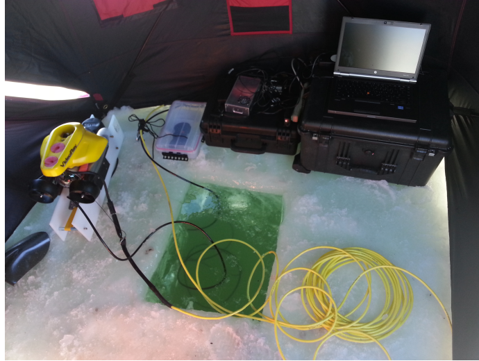
Figure 29: Lake John under-ice experimental testing setup and base station
