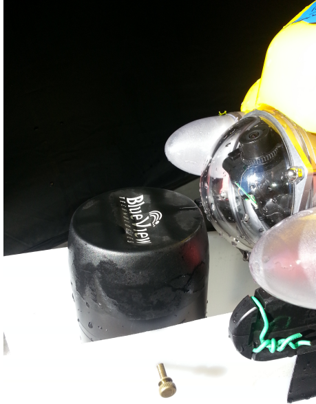
Figure 30: Videoray sonar and video sensors in 90 degree straight-up configuration
