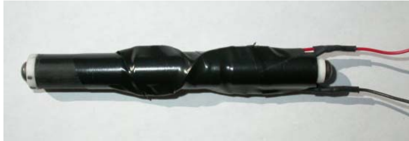
Figure 2.4: Three EPCOS stacks
