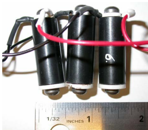
Figure 5.4: EPCOS PZT Array
