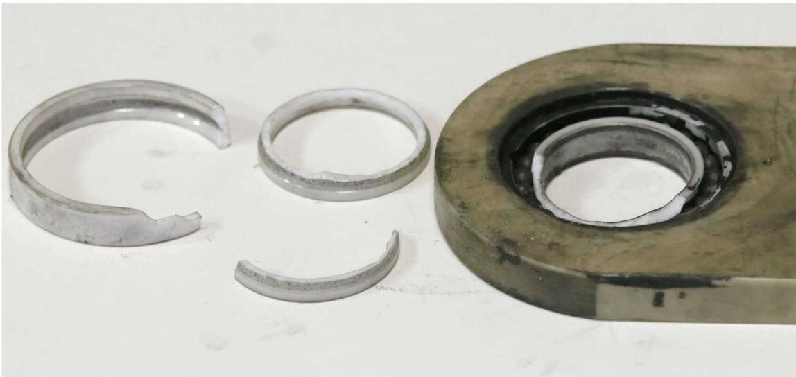
**Figure 16:** Zirconia ( $ZrO_2$ ) ball bearing failure
