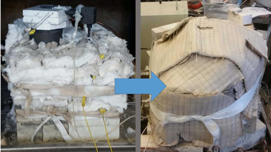
**Figure 40:** Insulation process for experiments above 1000°C
