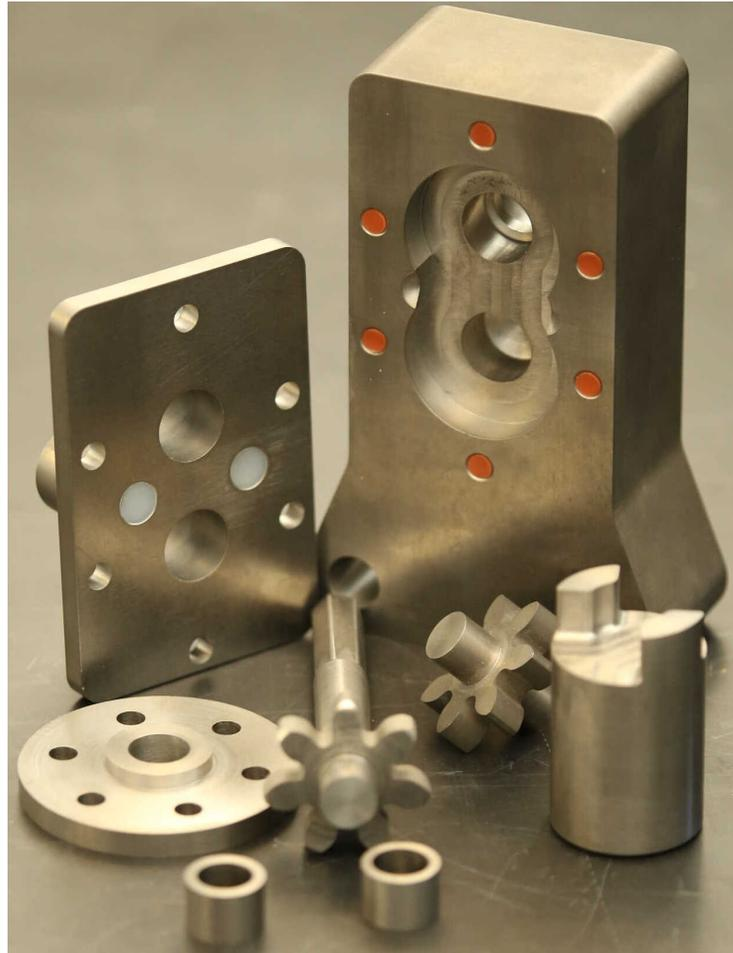
**Figure 6:** Tungsten external gear pump
