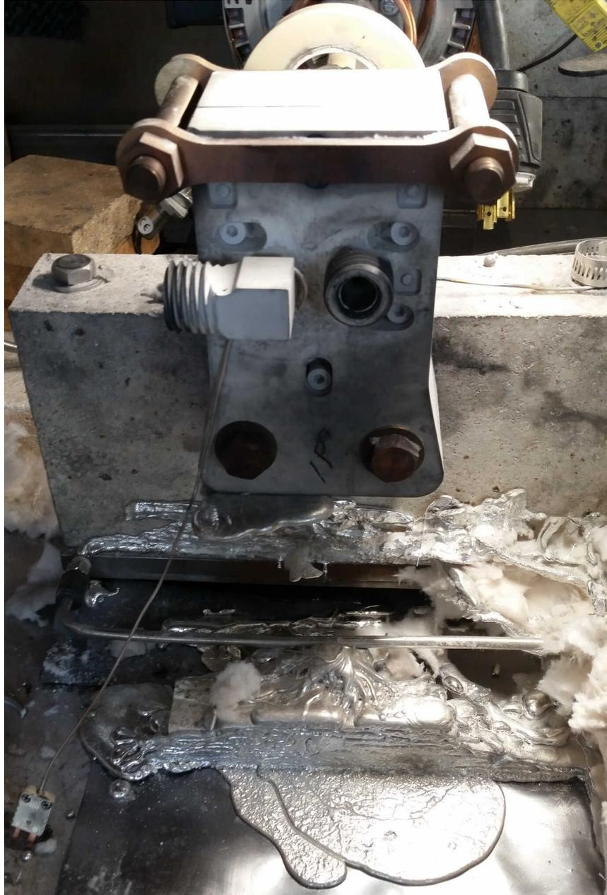
**Figure 50:** Leak caused by loosening of pump face seal bolts from thermal expansion
