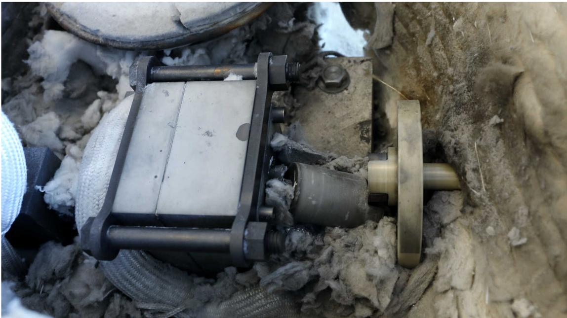
**Figure 54:** Pump failure caused by phase transformation and misalignment induced stress in the  $ZrO_2$  bearing. The Shapal pump shaft has visibly failed, but this was preceded by failure of the bearing.
