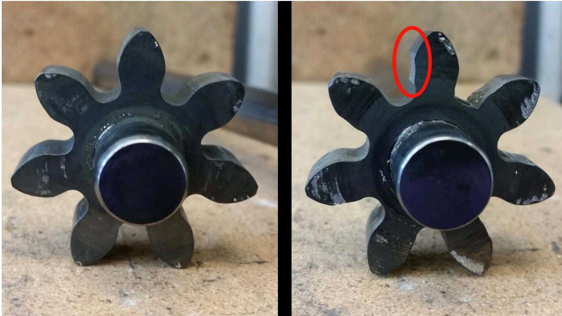
**Figure 47:** Corrosion on Inconel 625 gear teeth after scratching
