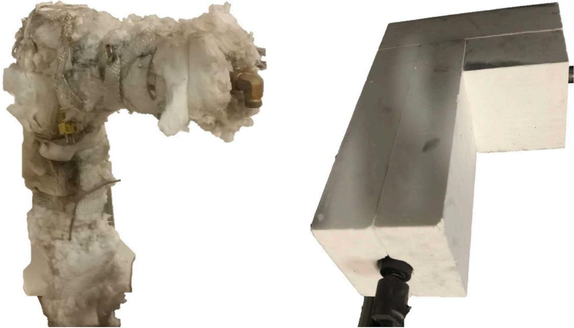
**Figure 39:** Alumina blanket (left) and rigid (right) insulation
