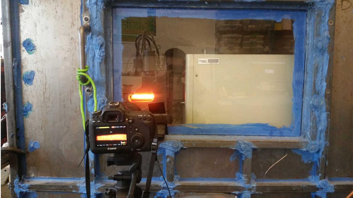
**Figure 45:** Chamber view including seals and visual flowmeter port
