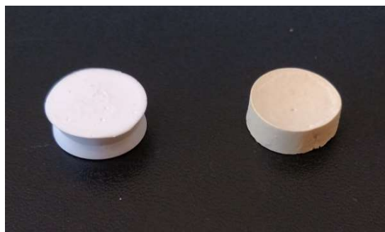
Figure 32 Example of cured polyHIPE samples, without MOF on the left, with MOF on the right. Samples shown are ~1/2” in diameter.
