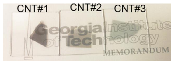
Figure 3.31 Optical images for the three CNT films used in this research. CNT#1 and CNT#1 are films of metallic nanotubes with thickness of 135 nm and 38 nm, respectively. CNT#3 is a semiconducting film with 30 nm thickness.
