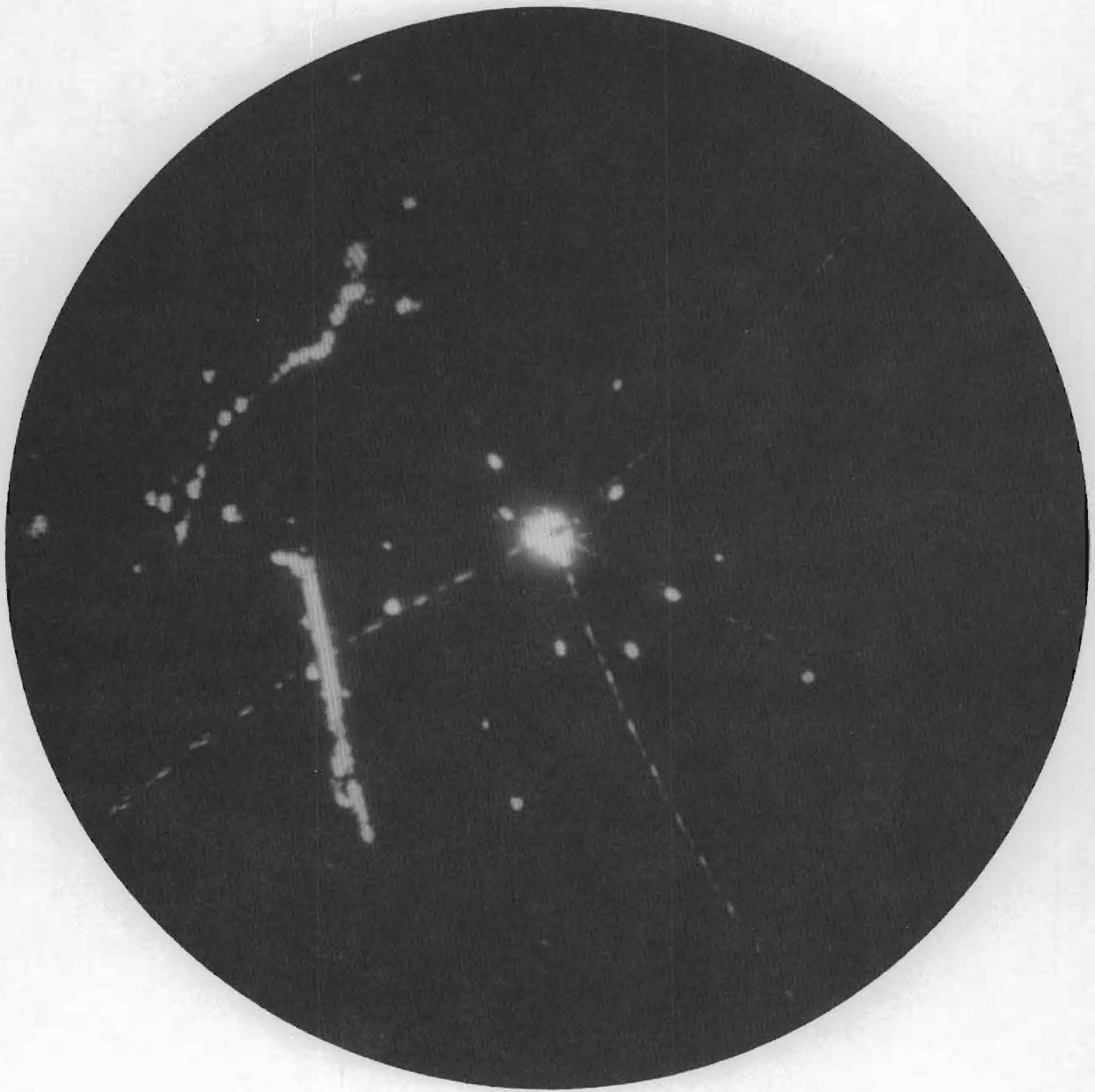
Figure 6. Radar display illustrating partial (about 50 per cent) minor-lobe interference. The range sweep is about 25 miles.
