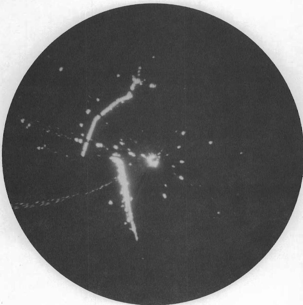
Figure 7. Radar display illustrating main-lobe interference. The range sweep is about 25 miles.
