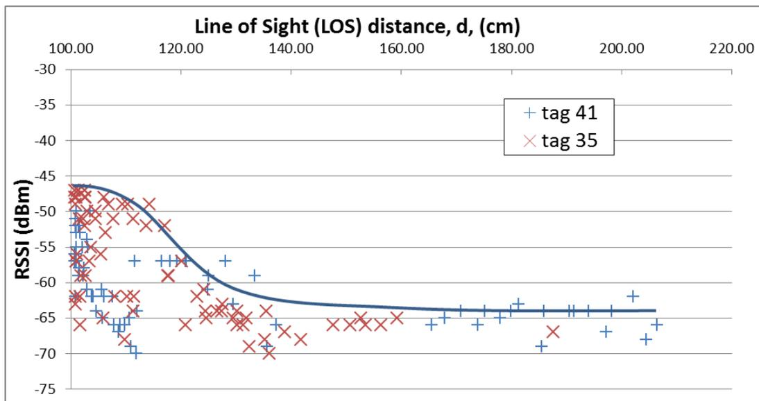
Figure 4.5: RSSI with Respect to Line of Sight Distance
