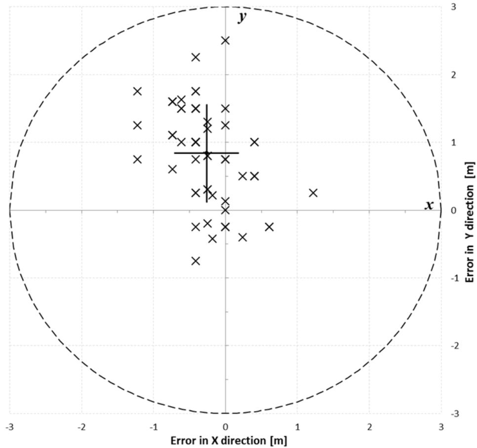
Figure 4.11: Scatter Plot of the Localization Error
