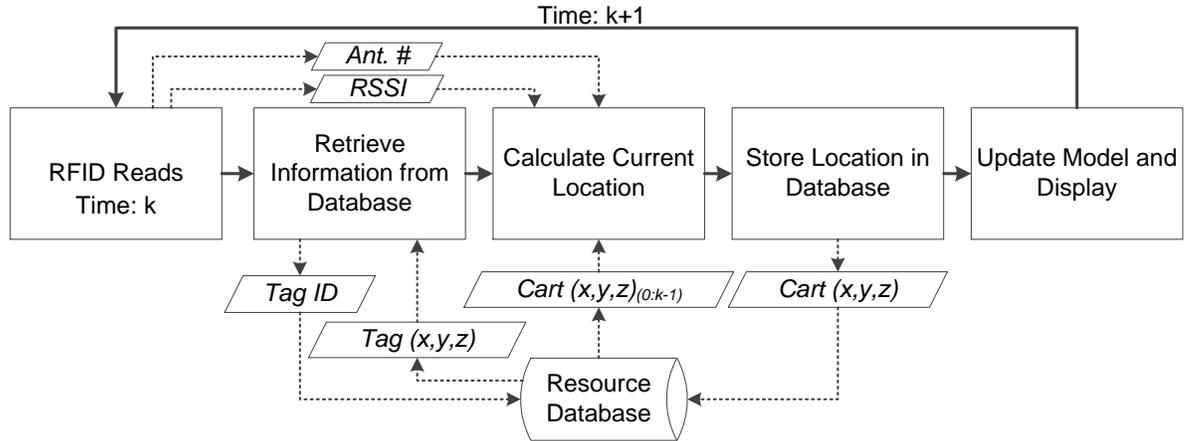
Figure 3.3: Process Flow of Localization and Visualization Algorithm
