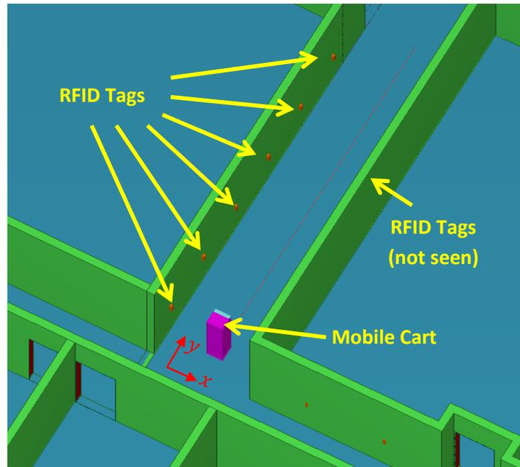
Figure 4.8: Facility Model with RFID Tags and Mobile Cart
