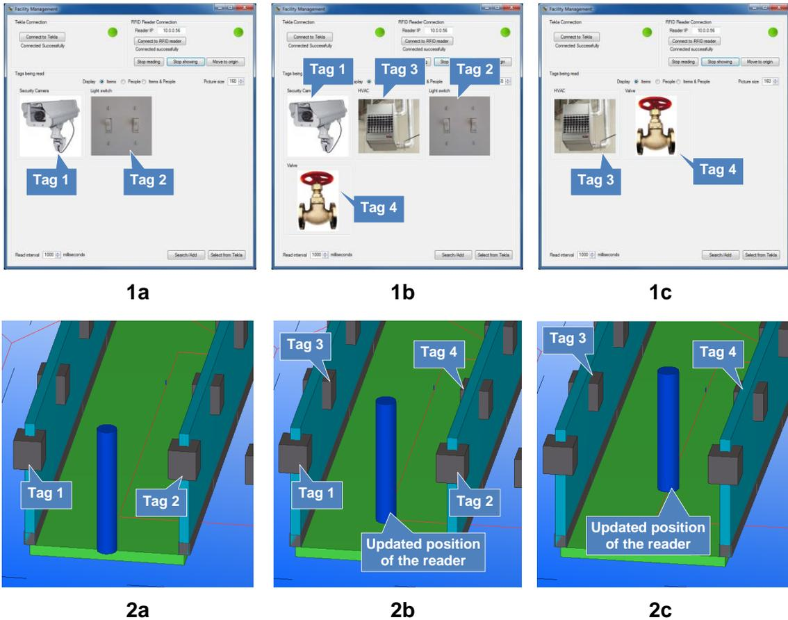
Figure 4.7: Demonstration of Localization: (1a) Tags 1 and 2 Being Read; (2a) Localization Based on Tag Reads 1 and 2; (1b) Tags 1, 2, 3 and 4 Being Read; (2b) Localization Based on Tag Reads 1, 2, 3, and 4; (1c) Tags 3 and 4 Being Read; and (2c) Localization Based on Tag Reads 3 and 4
