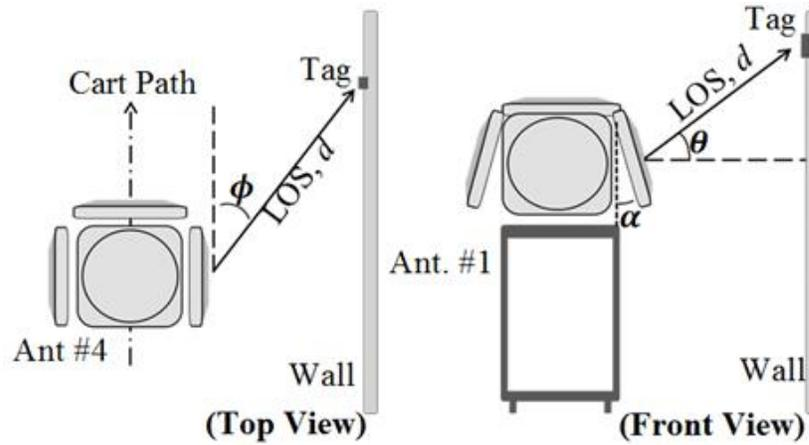
Figure 4.4: Line of Sight (LOS) of the Antennas Showing the Azimuth Angle, Phi (Left); and Elevation Angle, Theta (right)
