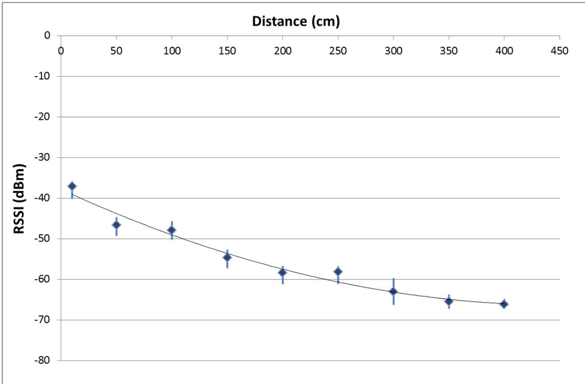
Figure 4.3: RSSI with Respect to Distance
