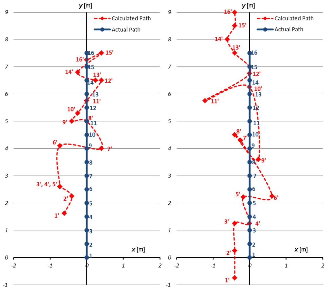
Figure 4.12: Calculated Path Versus Actual Path for Trial 1 (left) and Trial 2 (right)
