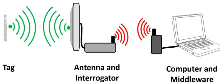
Figure 2.3: Wireless RFID system
