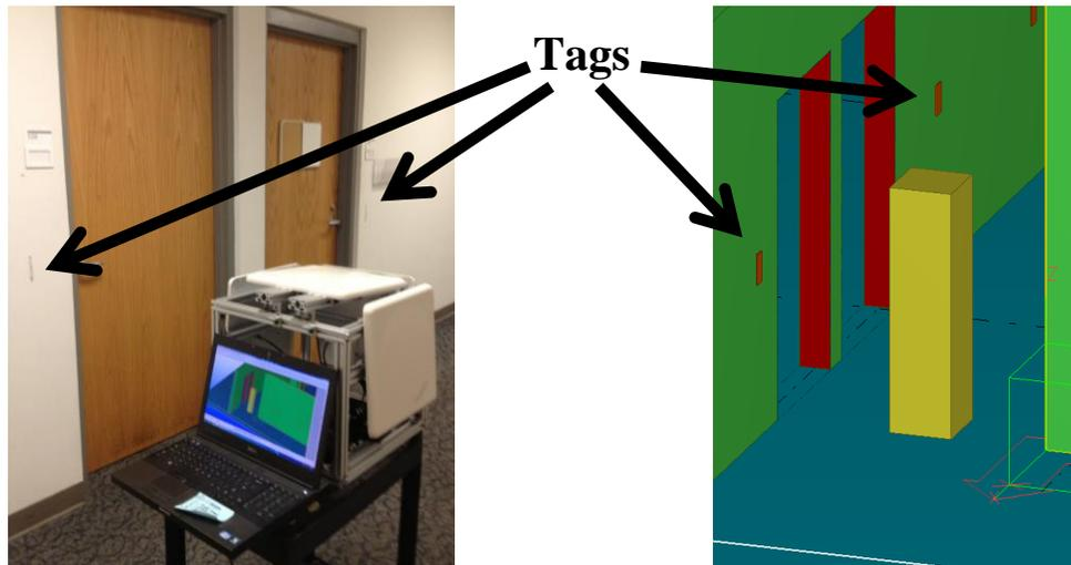
Figure 4.9: Actual location of Cart (left) and Display in BIM Model (right)
