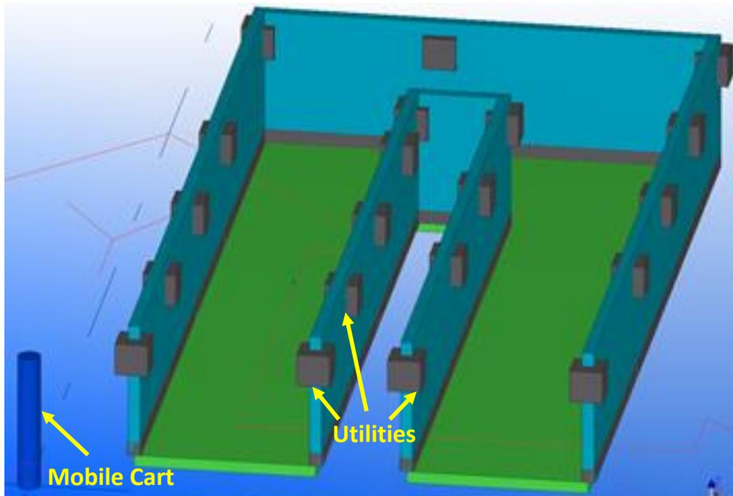
Figure 4.6: Tekla Model of Corridor and Utilities
