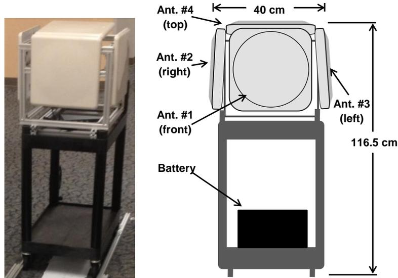
Figure 3.2: Mobile Cart (left) and Front View with Dimensions (right)
