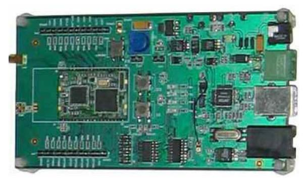
Figure 7-11: The prototype board contains the Cirronet-Zigbee chip, a DC voltage regulator circuit providing 3V and 5V, and a serial communications circuit for USB connection. The remainder of the components are connections for easy prototype development.
