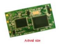
Figure 7-10: The ZMN2400HP wireless chip is used for sensor communications over short distances.
