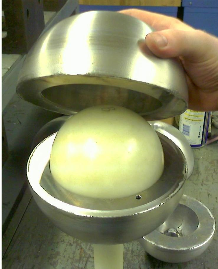
**Figure 14. The 5” spherical shells (large assembly) in early production stages. The first locking lip can be seen cut into the surface.**
