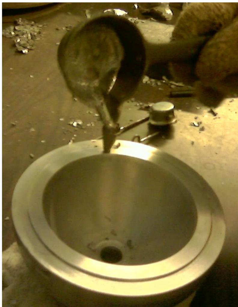
**Figure 15. Smelting lead and ladling it into the shell.**
