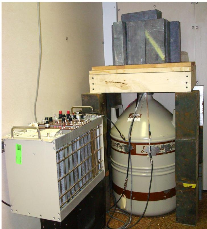
**Figure 8. HPGe detector setup with lead shielding cave and NIM modules for running the detector.**
