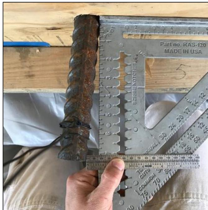
**Figure 17. Dowel Bar Horizontal Alignment Measurement**
