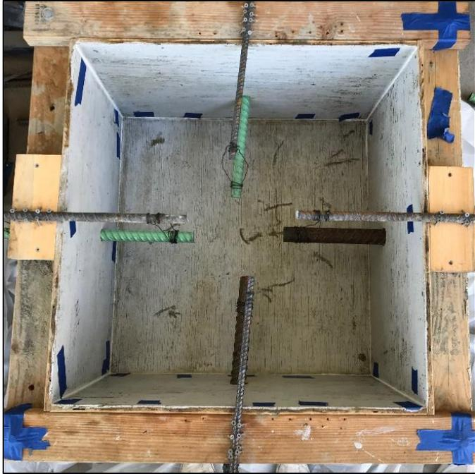
**Figure 46. Dowel Bar Sample Image Before Casting**
