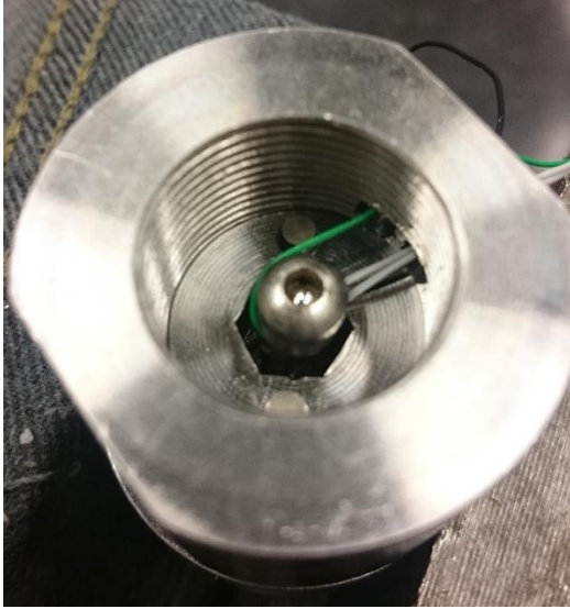
Figure B.18: Internal view of HPEH7-1 during assembly, with single crystal in place, dowel pins in place, male spherical bearing on single crystal, and wires from electrodes and strain gauge wired through ports.
