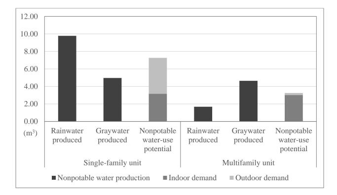
Figure 5. Non-potable water production and consumption potential per household – Lindbergh, 2018
