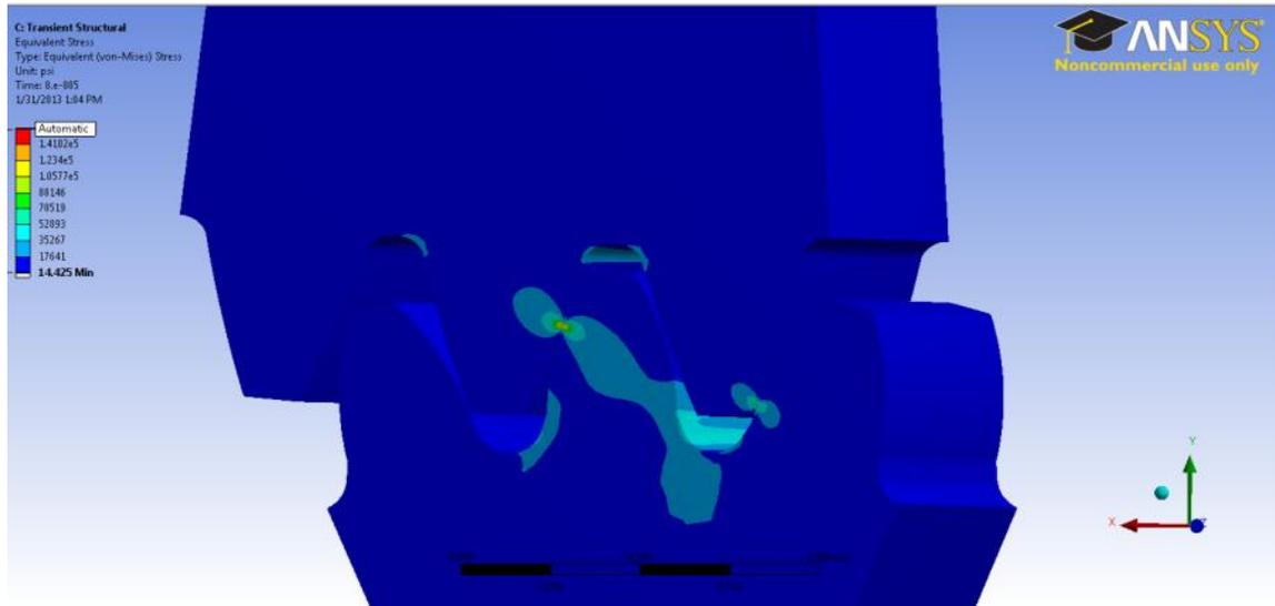
Figure 127. von-Mises stress contours for transient analysis
