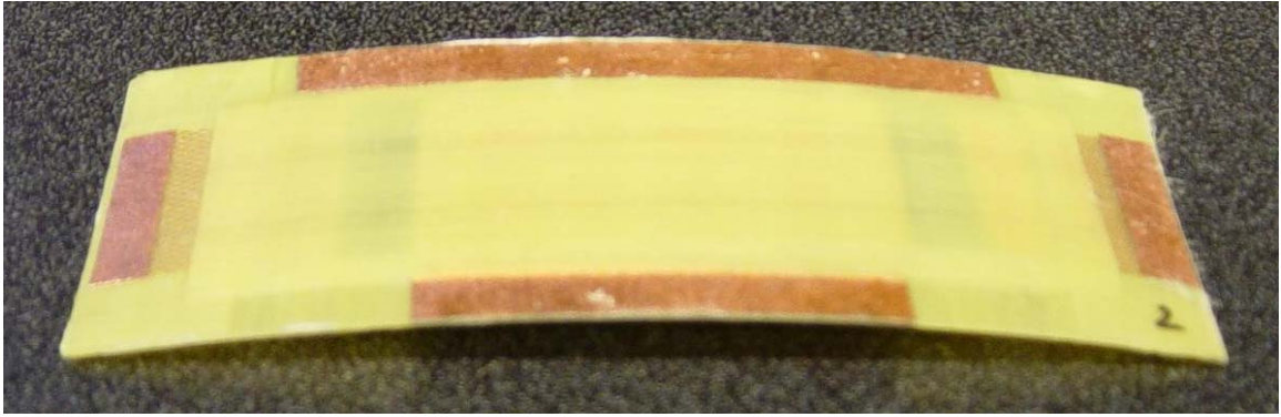
Figure 3.8. GEPAC (after curing)
