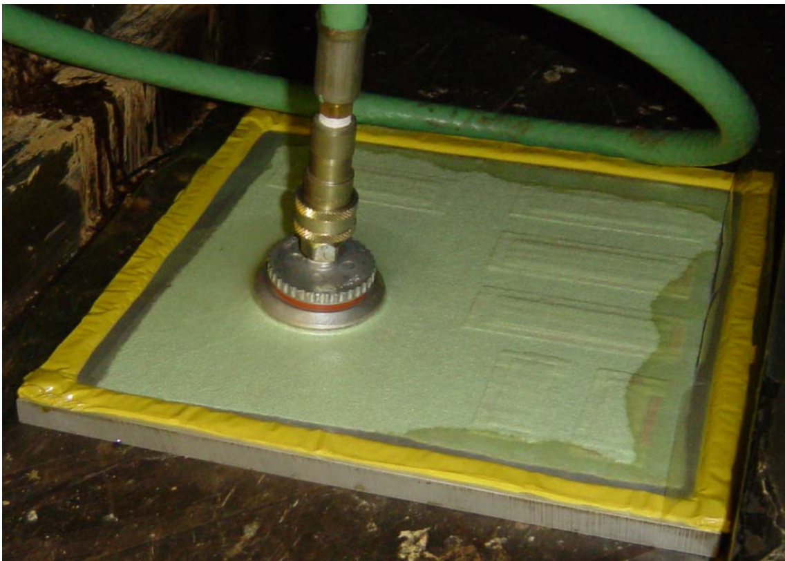
Figure 3.7. Mold in the autoclave right after the cure cycle
