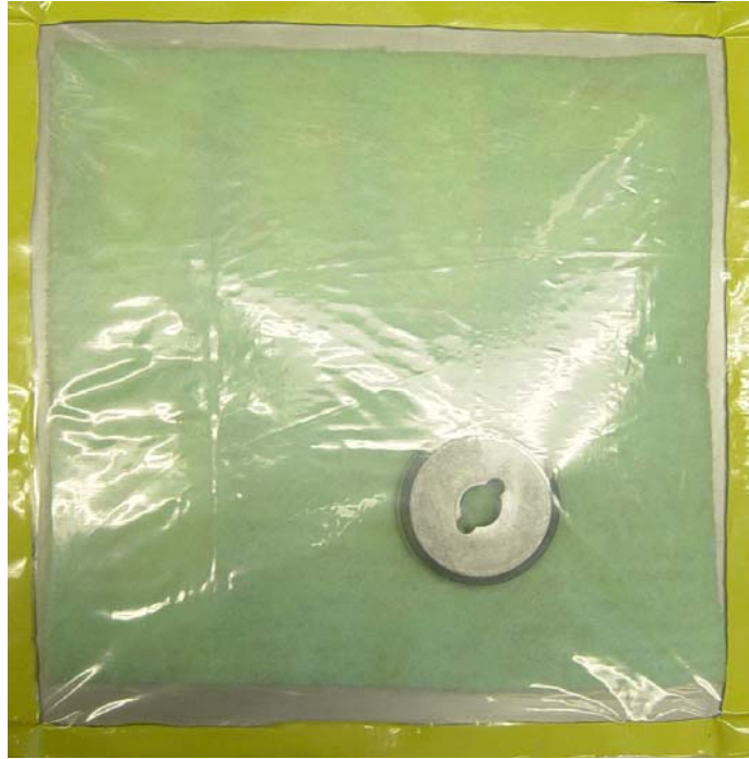
Figure 3.5. Mold for the curing of GEPAC
