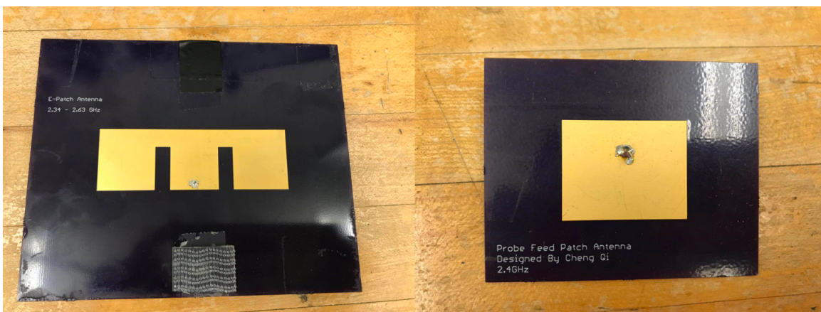
Figure 30– Tx Antenna (Left) [18] and Reference Antenna (Right) for 2.4GHz
