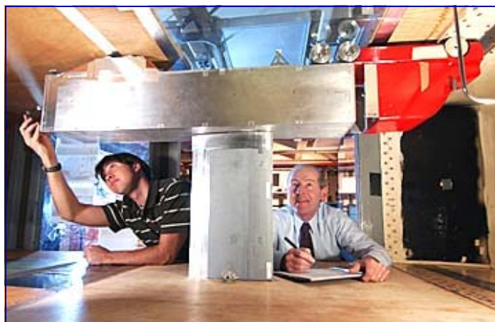
Researcher Robert Englar (right) and co-op student Daniel Hegeman adjust blowing slots on a model truck inverted in GTRI's low-speed wind tunnel. The testing helped assess the value of fuel-saving improvements.
