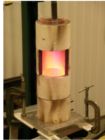
Figure 1. Schematic of the SPRF combustor and photograph of the combustor operating on natural gas.
