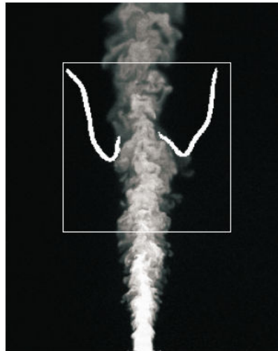
Figure 3. Fuel concentration distribution in a lifted turbulent jet flame from Mungal et al. [20] with the flame location superimposed on it.
