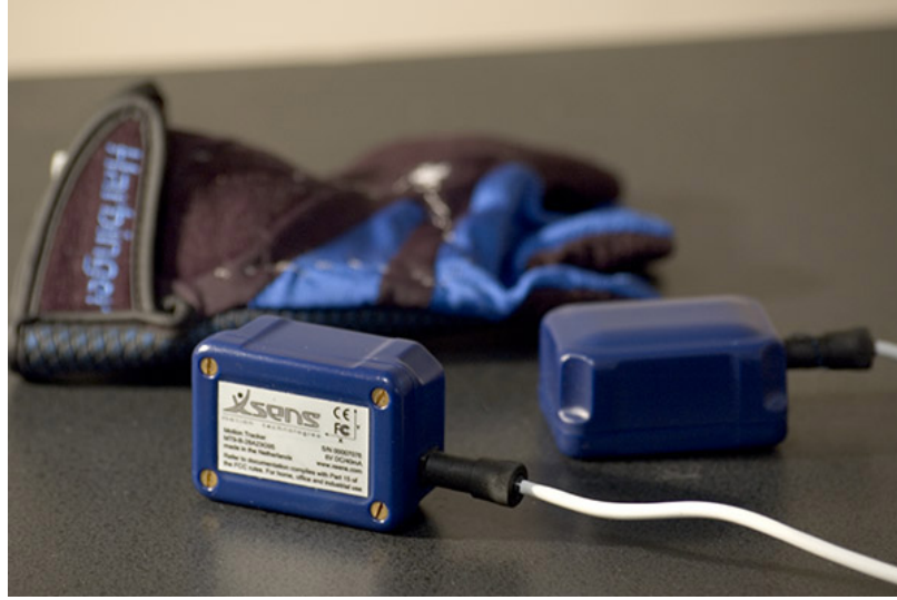
Figure 26: Two XSens MT9 inertial sensors and a modified glove used to mount a sensor on a subject’s wrist. The MT9 measures acceleration and rate-of-rotation in three axes at 100Hz.
