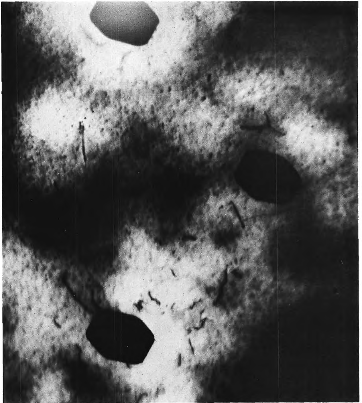
Figure 25. Transmission Electron Micrograph of \text{UO}_2 -W Composite Showing Hexagonal Cross Section of Several W Fibers. About 25,000X.
