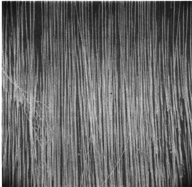
Figure 37. Scanning Electron Micrograph of Longitudinal Section of a \text{UO}_2 -W Composite Showing W Fiber Continuity. 550X.
