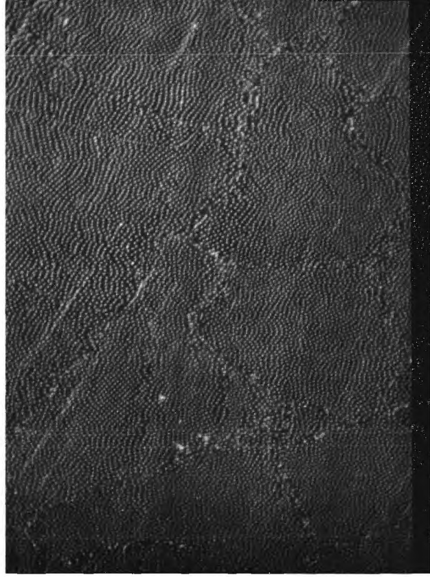
Figure 39. Transverse Section of a Stabilized ZrO 2 -W Composite. Dark Field, 200X.
