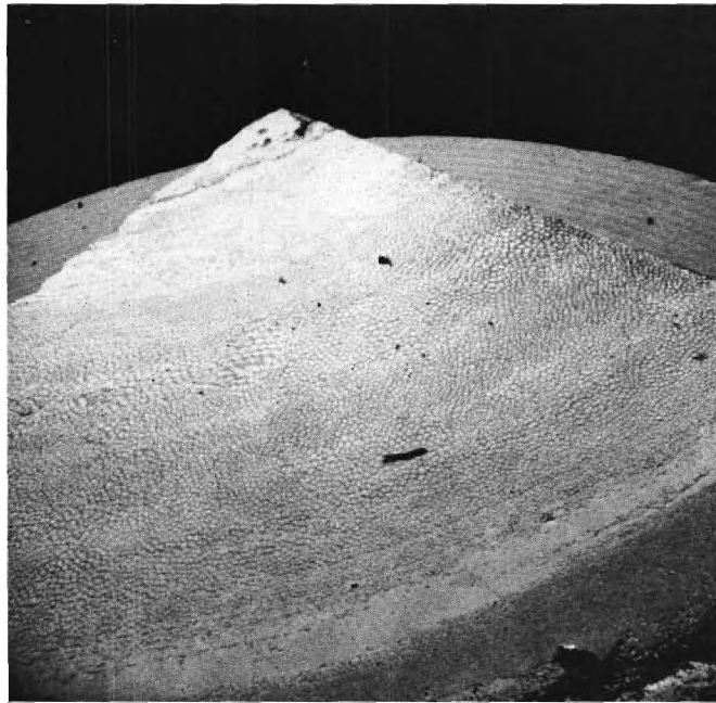
Figure 11. Scanning Electron Micrograph of \text{UO}_2 -W Composite Showing Contrast Obtained at Low Magnification When Backscattered Electron Mode Is Utilized. 20X.
