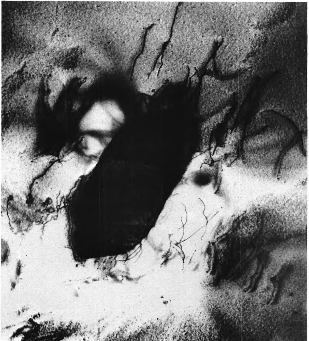
Figure 28. High Voltage Transmission Electron Micrograph of Tungsten Fiber in \text{UO}_2 Matrix After Sample Thinning by Ion Etching. Fiber Is Viewed at Approximately 45^\circ Off Fiber Axis. 50,000X.
