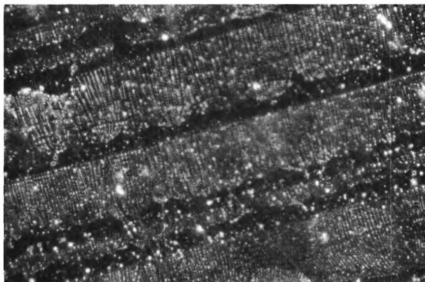
Figure 32. Longitudinal Section of \text{UO}_2 -W Composite, Containing 5 Weight Percent W, Exhibiting "Banding". Sample Was Grown Without Rotation With the Growth Direction From the Bottom to the Top of the Figure. Dark Field, 600X.
