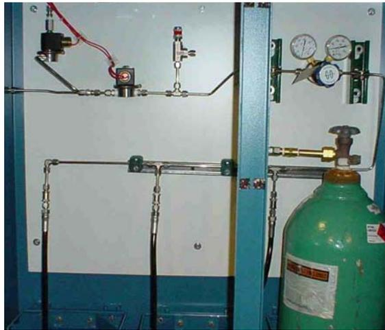
**Figure 7: Bottle Valving and Controls for Hydrogen and Carbon Monoxide**
