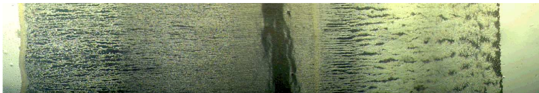
Figure 42: Microscope image of migrated silver on PEDOT:PSS resistor. A DC-voltage of 500 V was applied for 3 hours before the picture was taken. The anode is to the right.
