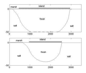
Figure 2. Position of the interface along crosssections A—A' (top) and B—B' (bottom); vertical scale exaggerated.
