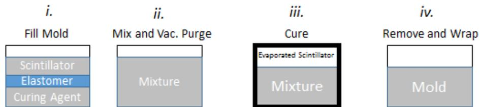
Figure 26. Solidification procedure step diagram.
