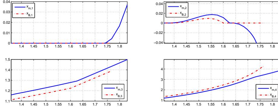
Figure 30: Second sliding on  $\Sigma$ : moments trajectory evolves properly, whereas bilinear trajectory develops a singularity after passing through a first order exit point.
