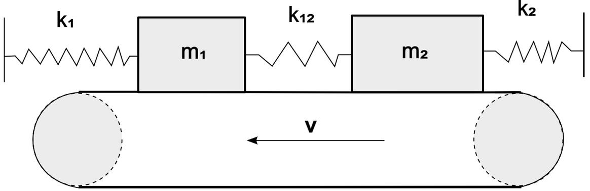
Figure 1: Stick-slip 2 block mechanical system described by (1.1.1).
