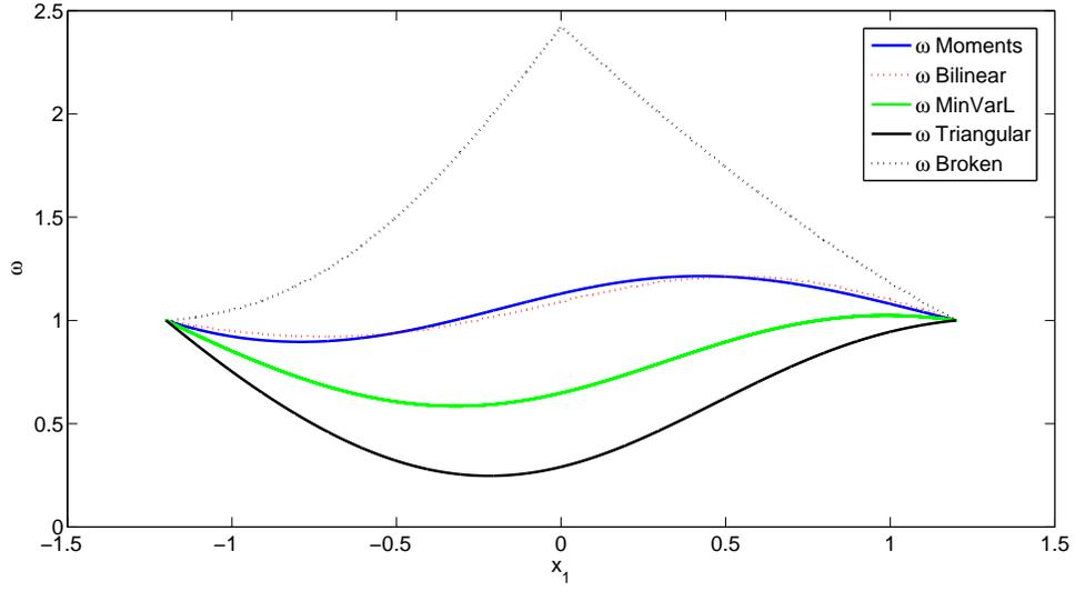
Figure 35: Orbital equivalence factors  $\omega$  for moments, bilinear, triangular, broken-line, and minimum variation with respect to  $\lambda$ .
