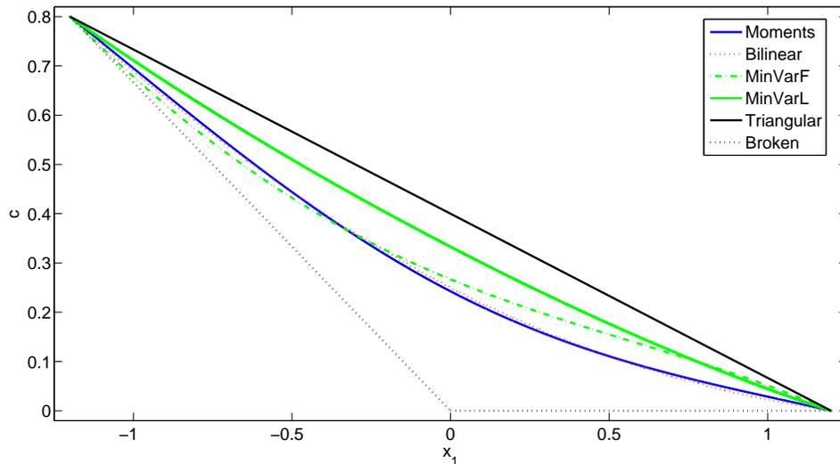
Figure 33: Admissible region  $(x_1, c)$  and moments, bilinear, triangular, broken-line, and minimum variation solutions of  $c$ .
