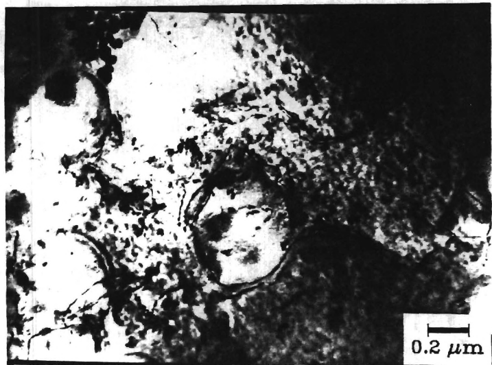
Fig. 27 - TEM micrograph showing dislocation by-pass of large \gamma' particle.
