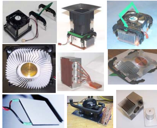
Figure 8-16 - Examples of CPU Heat Sink Designs
