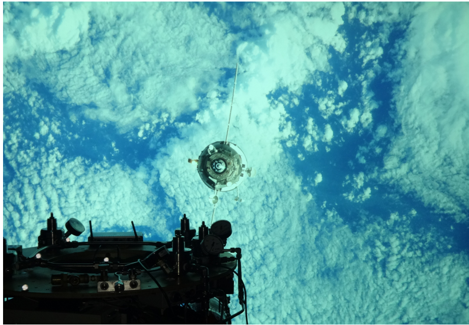
Figure 3 A large projection screen is used to simulate virtual Earth orbit scenarios. Part of the ASTROS upper stage platform is visible at the left bottom corner.
