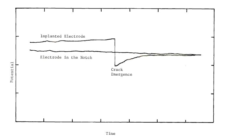
Fig. 14. Potential Variation vs. Time as Measured by the Implanted Electrode and an Electrode in the Notch.
