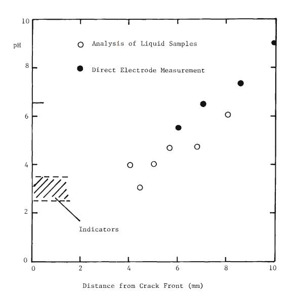
Fig. 9. Results of pH Measurements Using Various Techniques.
