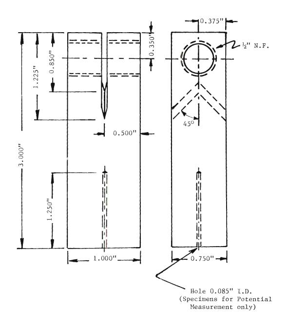
Fig. 1. SCC Specimen for the Determination of Electrochemical Conditions within cracks.
