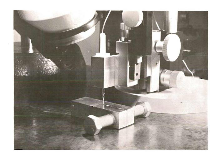
Fig. 4. Experimental Setup for Application of Microprobes in Cracks (Detail).
