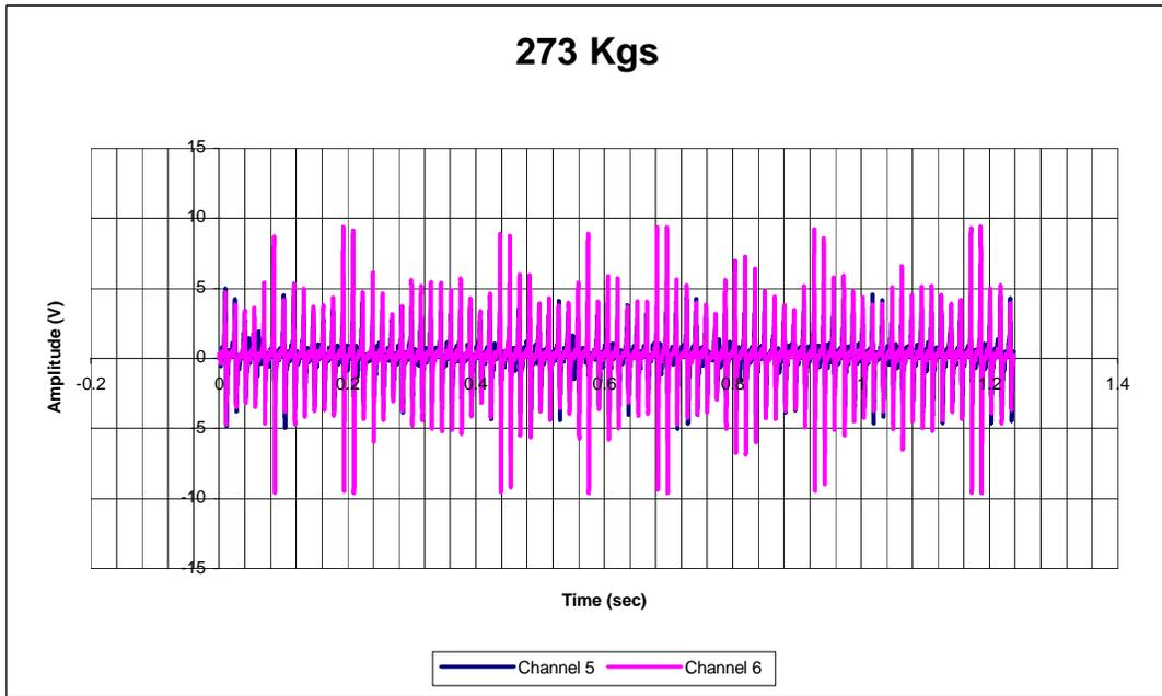
**Figure 52. 273Kg Channel 5-6 five cage rotations captured**
