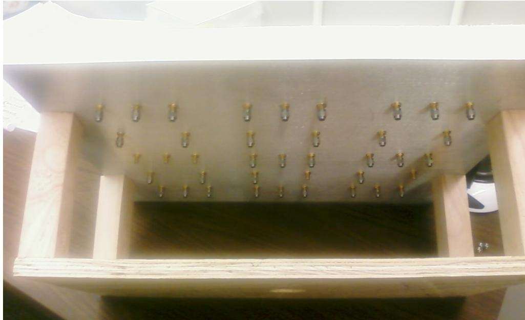
**Figure 4.11 Side view of the fabricated dual-band array showing the foam layer, the SMA ports and the wooden frame.**
