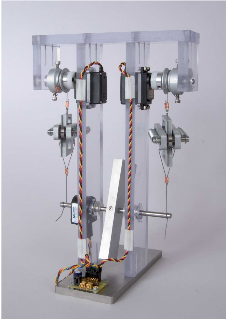
Figure 13: The single degree of freedom device with antagonistic, series-elastic actuation.
