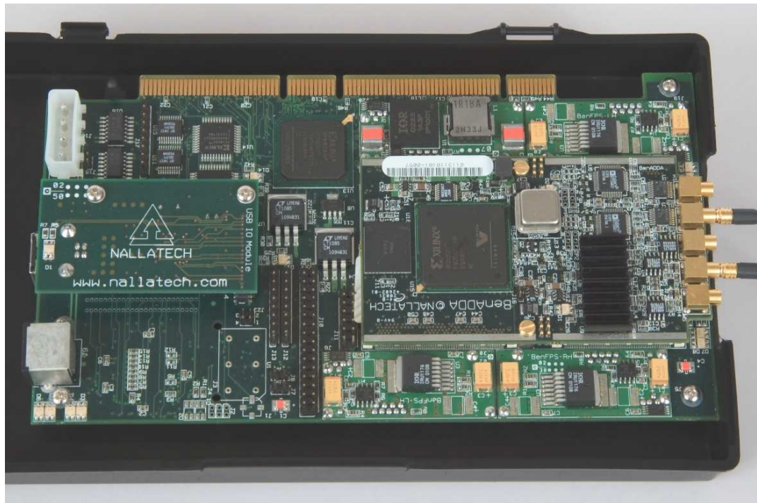
Figure 14: The Xtreme DSP Development Kit, an FPGA-based controller used for the system.
