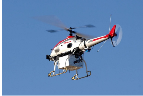
Figure 3: Yamaha RMAX-based research UAV utilized for this effort, 3130 mm main rotor
