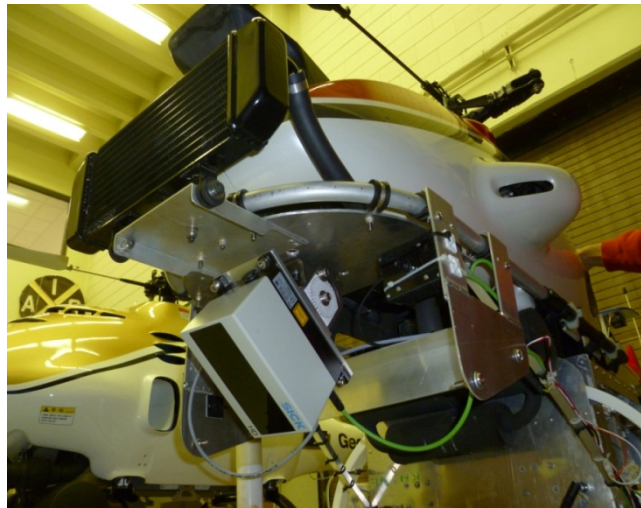
Figure 4: Sick LD-MRS Laser scanner mounted under the nose of the aircraft, able to see down and forward (sensor rotated 90 degrees in roll, 40 degrees nose down pitch)
