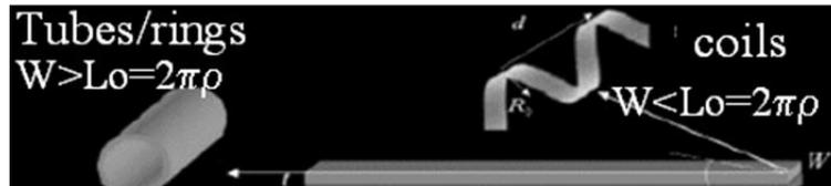
**Figure 1-7: Schematic of a strained bilayer film folding into a tube when  $W$  is large, but into a coil when  $W$  is small. The arrows indicate the folding direction[39]**
