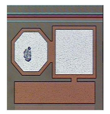
• Double bond pads on the device die. One pad is used for temporary packaging for burn-in purpose and the other for actual application wire bonding.
