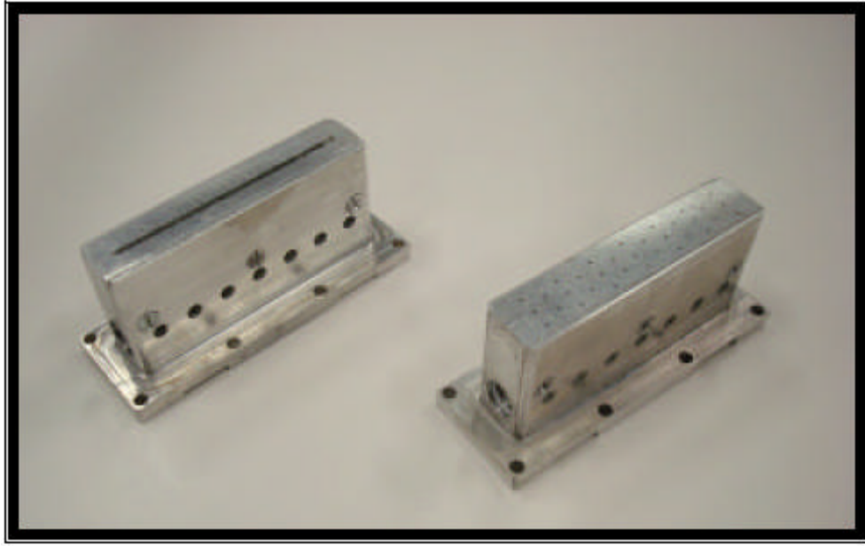
Figure 2.4: Photograph of the manufactured inner cartridges. The outlet port is visible near the bottom of the side of both cartridges.
