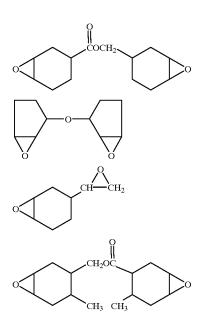
A distinguishing feature of many of the cycloaliphatic epoxides is the location of the epoxy group(s) on a ring structure rather than on an aliphatic side chain. Generally, the cycloaliphatic epoxide particularly useful in this invenof:
