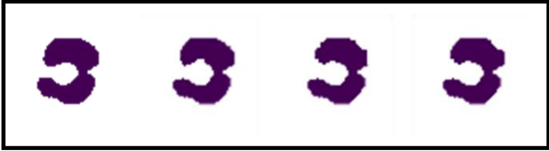
Figure 4.6 – Results from Evolution Strategy for optimal plasmonic geometry to yield maximal SHG response.
