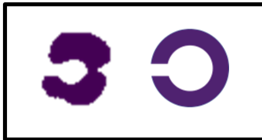
Figure 4.7 – Optimized structure and split ring resonator (SRR) with similar parameters. The optimized structure had a significantly higher second-harmonic nonlinear optical response as compared to the split ring resonator.
