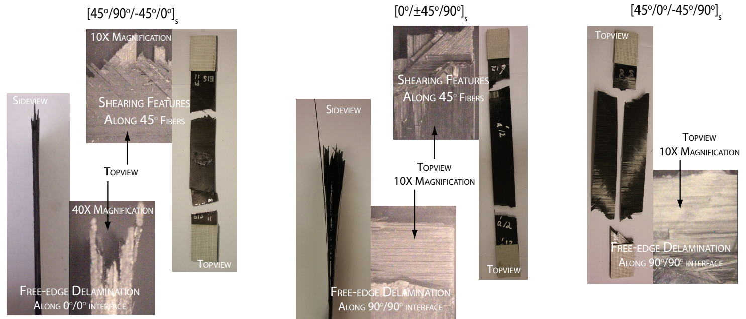
Figure 40: Quasi-static failure mode comparison for IM7/8551-7 (IM7/8551-7) [45/90/-45/0]_s , [0/\pm 45/90]_s and [45/0/-45/90]_s Adherend fracture sketch taken from Heslehurst and Hart-Smith [49]
