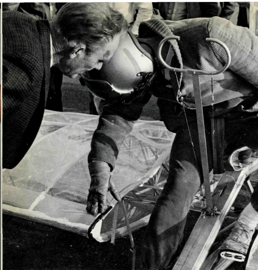
Richie inspects the damage to the wing at the end of the unfortunate flight of the MPA-1. Richie and other Tech undergraduates are now rebuilding for another try.
