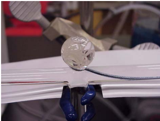
Figures 17 (left) and 18 (right). Two SMP coils deployed in glass aneurysm under simulated blood flow conditions (side view and end view).
