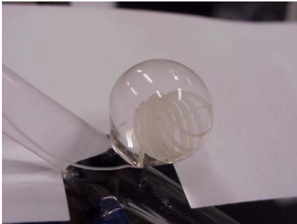
Figures 15 (left) and 16 (right). One SMP coil deployed in glass aneurysm under simulated blood flow conditions (top view and side view).
