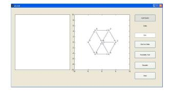
Fig. 1. A graphical program derives  $\mathbb{G}$  from a set of desired positions entered by a user, representing a desired formation. This program also simulates the network in the left plotting area.
