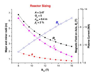
Fig. 4 Various reactor parameters  $(R_0, a, B_0, I_p)$  vs. the maximum toroidal field at the coil,  $B_{TF}$ , for a set of fixed shape and performance parameters.
