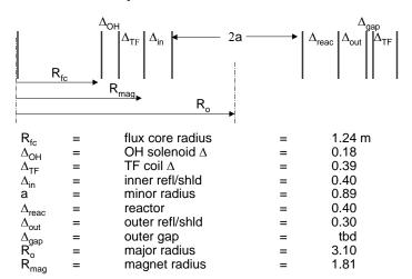
Note: refl/shld includes first wall, reflector, shield, and vacuum vessel
