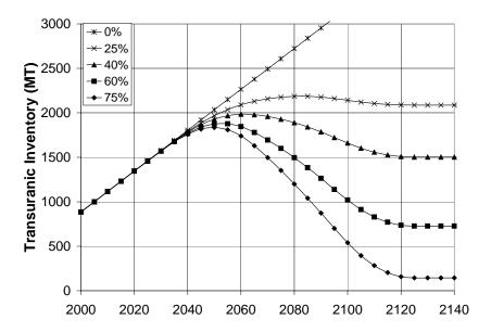
Fig. 10 Estimated Future Transuranic Inventory as a Function of FTWR Availability. (0% corresponds to the Once Through Cycle without FTWRs)
