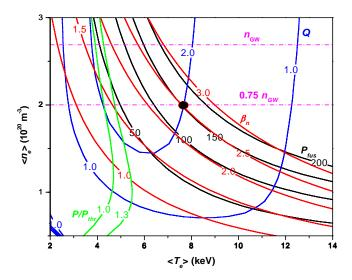
Fig. 5 POPCON Plot for the reference design of the fusion neutron source. Contours of constant fusion power,  $Q_p$ , normalized beta and  $P_{sep}$  /  $P_{LH}^{thr}$  ratio are shown. In addition, lines of constant  $\langle n_e \rangle$  /  $n_{GW}$  ratio are also shown. The reference operating point is marked by a solid circle.
