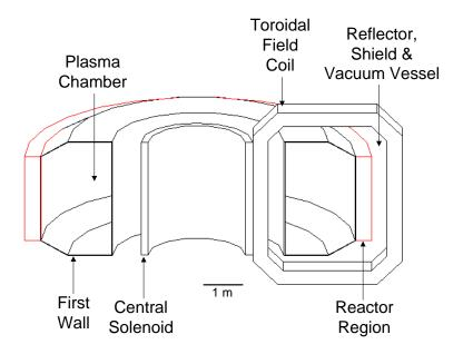
Fig. 1 Schematic of Geometric Configuration of FTWR
