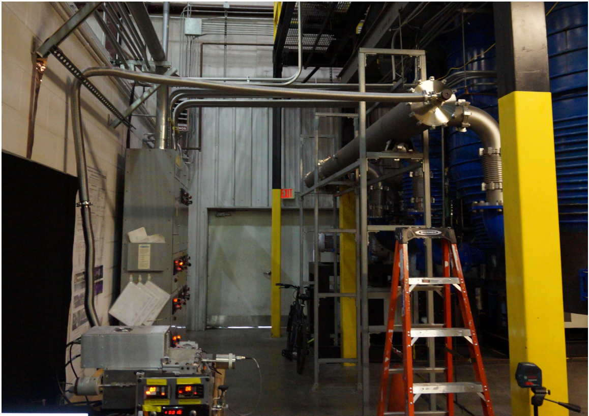
Figure 3.7: Experiment 2-inch stainless-steel vacuum gas exhaust line, with right angle isolation valve connection to VTF-1 manifold end-flange.
