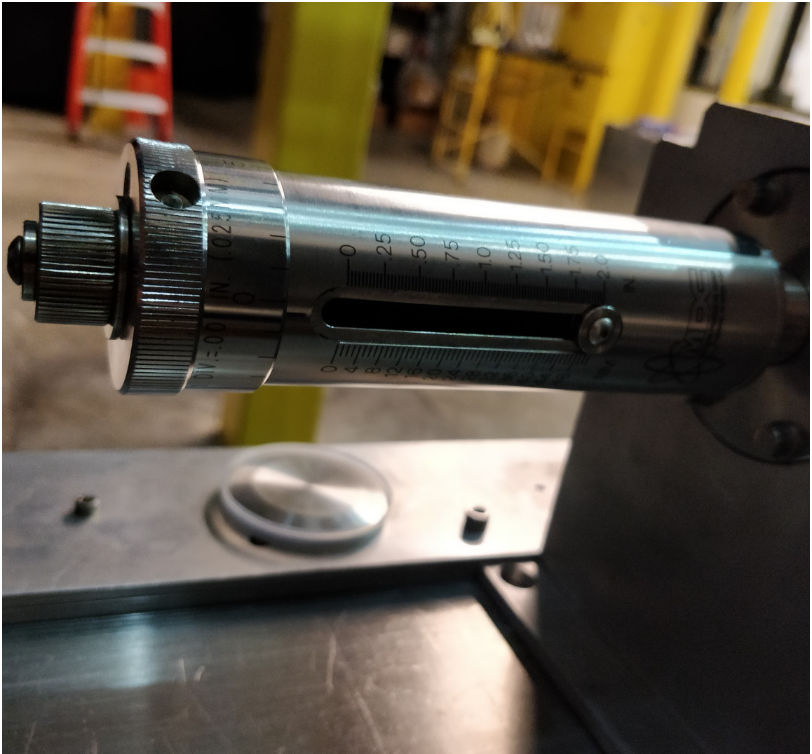
Figure 3.35: Linear micrometer feedthrough in fully extended position.
