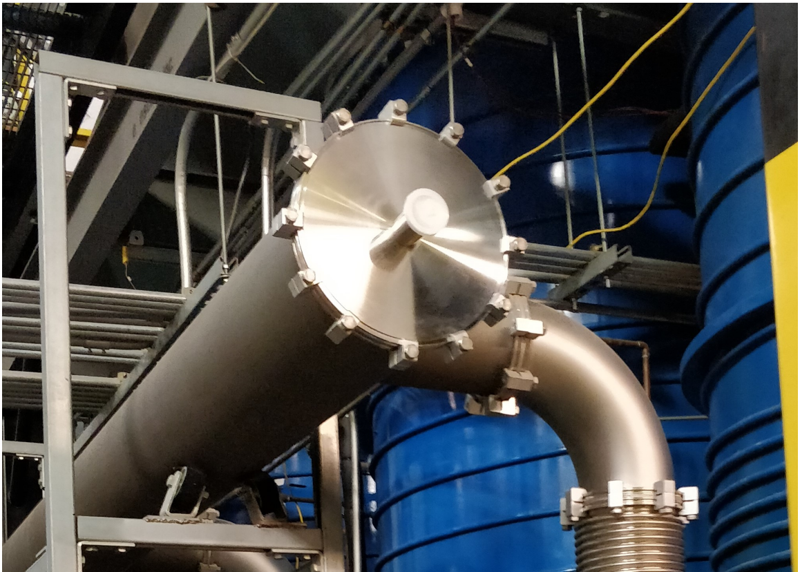
Figure 3.6: HPEPL VTF-1 pump manifold ISO-K 250 end flange with a custom adapter to KF40 flange installed.
