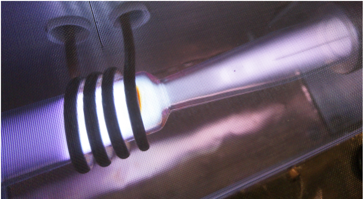
Figure 3.43: MEDTHERM thermocouple in supersonic plasma discharge. 800\text{ W} forward RF power, 9,300\text{ sccm Ar} ( 3\text{ V} ) gas mass flow rate. Measured temperature is approximately 1215\text{ K} .
