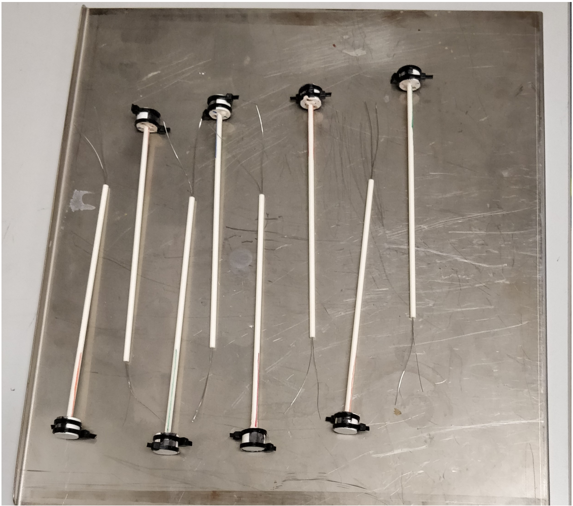
Figure 4.14: MHD model sub-assemblies on a plate for oven-curing.
