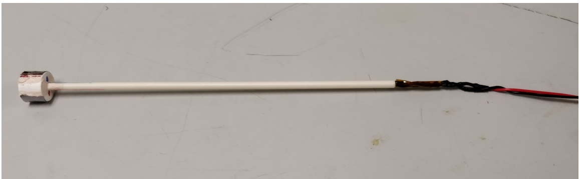
Figure 4.15: MHD model electrode wire solder extension to sliver-coated, Teflon insulated 24-AWG hookup wire for reduced lead resistance and model placement flexibility.
