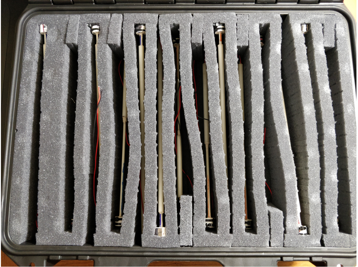
Figure 4.18: Full set of assembled 0 degree and 90 degree MHD energy generator model variations. N = 3 each for versions with embedded magnets and two control models without magnets. Total of 14 assembled models.
