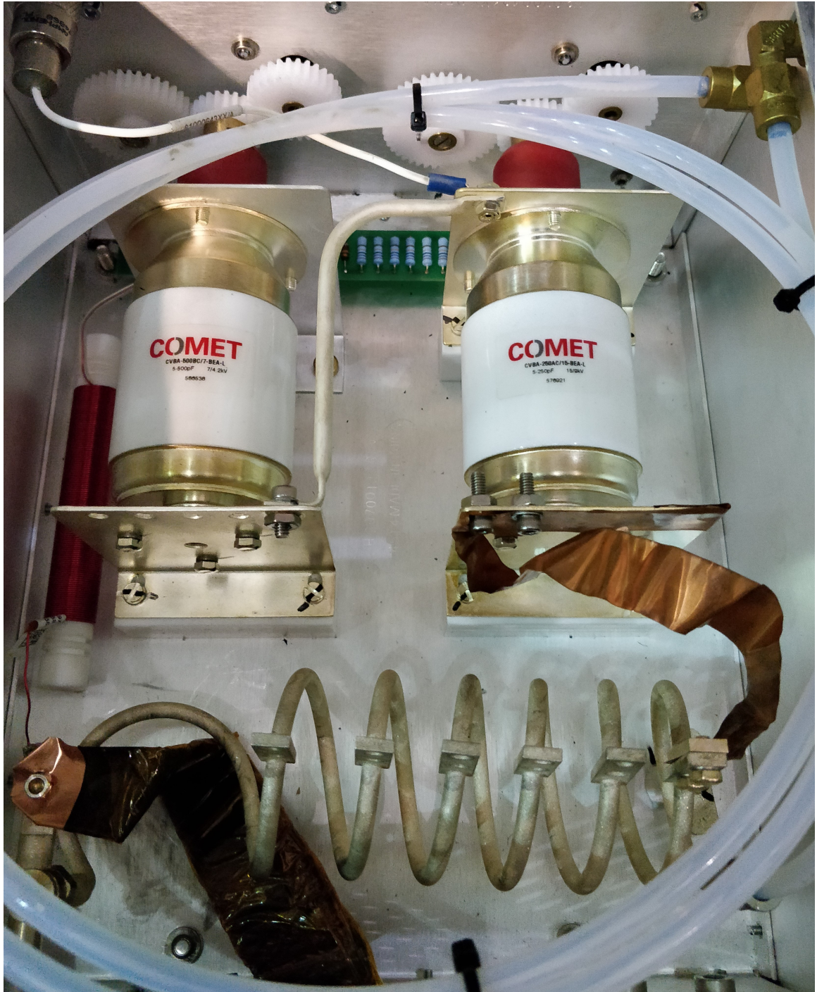
Figure 3.18: Advanced Energy model VM2715AW impedance matching network configuration with water-cooled 6-turn tune-coil connected for 6 active coils in L-match topology.
