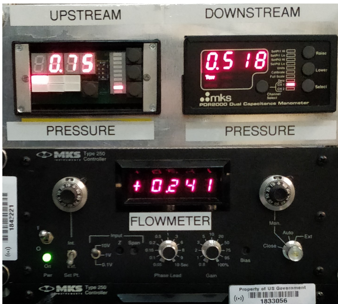
Figure 3.24: Test chamber gauge readouts. Upstream pressure is 0.75 Torr , downstream pressure is 0.518 Torr , and mass-flow rate readout is 0.241 V , as described in section 3.1.2.
