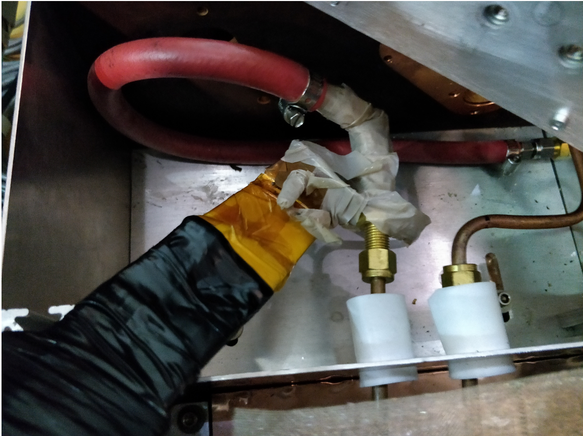
Figure 3.19: Thin copper strap connection between the matching network output and water-cooled copper RF antenna coil.
