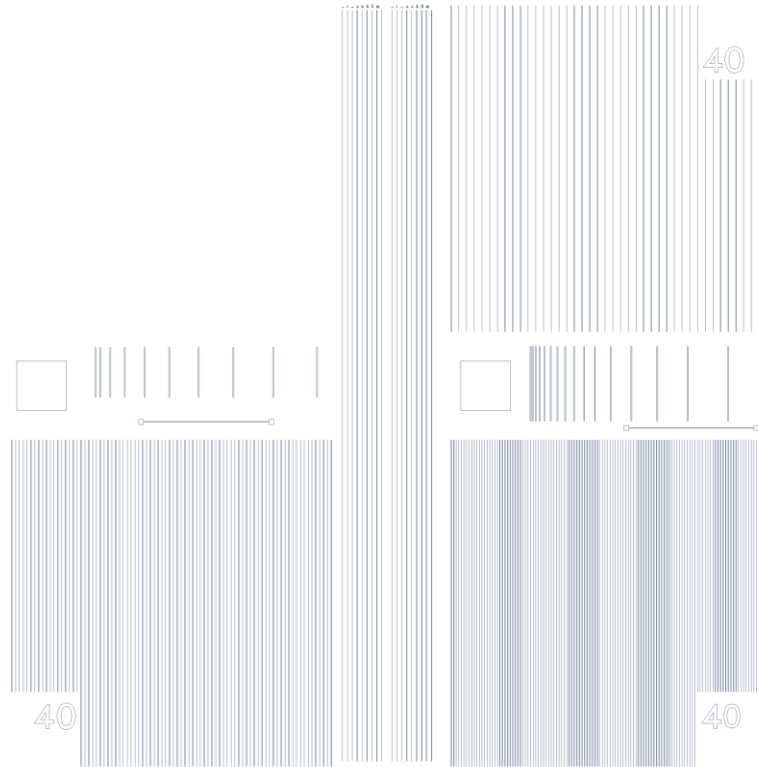
Figure 67: Test screen with different metal fractions and TLM patterns for metallized J_0 and contact resistance measurements.
