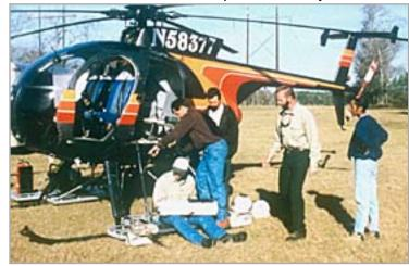
Researchers recently conducted a field test of their new power line crossarm inspection system that combines laser vibrometry and neural networks and allows workers to analyzes crossarm structural integrity from the air. The process drastically reduces costs, while also boosting accuracy. (300-dpi JPEG version - 489k)
