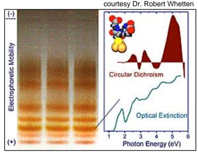
Experimental results show that tiny clusters of gold can show distinctly chiral optical properties. This figure shows electrophoretic separation of gold: glutathione cluster compounds, left, the circular dichroism effect observed, upper right, and optical extinction, lower right, of the third separated band. (300-dpi JPEG version - 529k)
