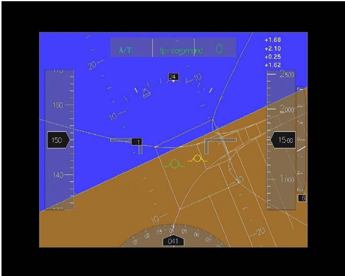
Figure 4- Tunnel in the sky primary flight display, in Command-FPV FCS format.
