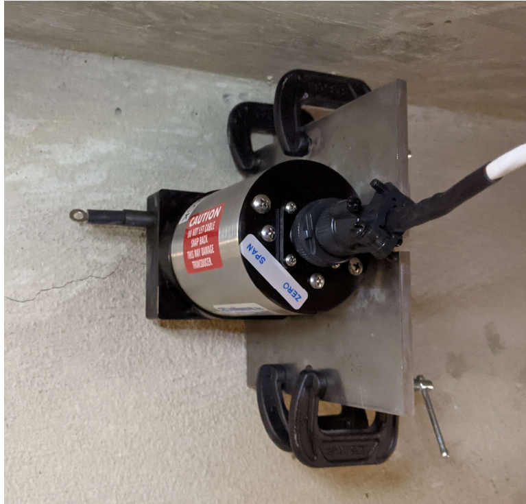
Figure 4.11: UniMeasure HX-P510 Series Linear Potentiometer
