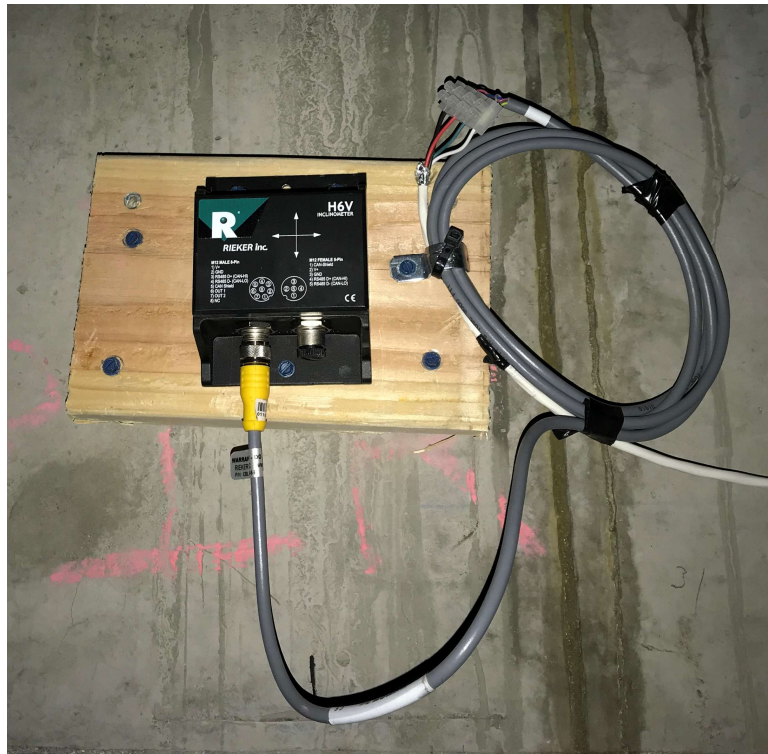
Figure 4.14: Reiker Flex Series H6 biaxial inclinometer installed a south face of pier diaphragm at Pier 2
