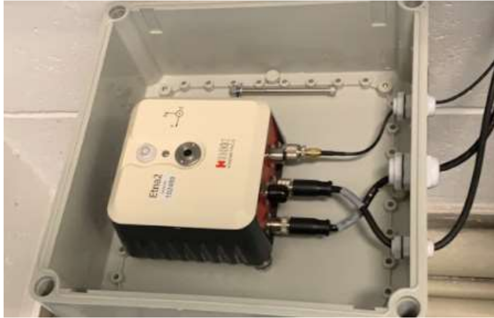
Figure 4.19: Kinematics ETNA 2 accelerograph and protective case
