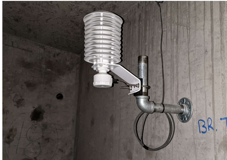
Figure 4.15: R.M. Young 41342 temperature probe located in Galena Creek Bridge
