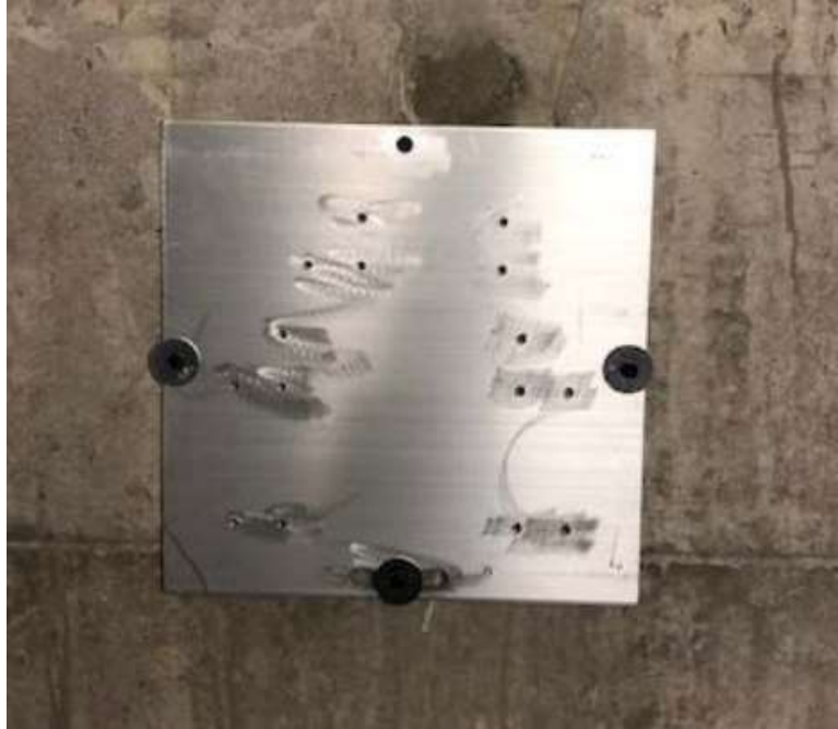
Figure 4.5: Aluminum plate for mounting accelerometers
