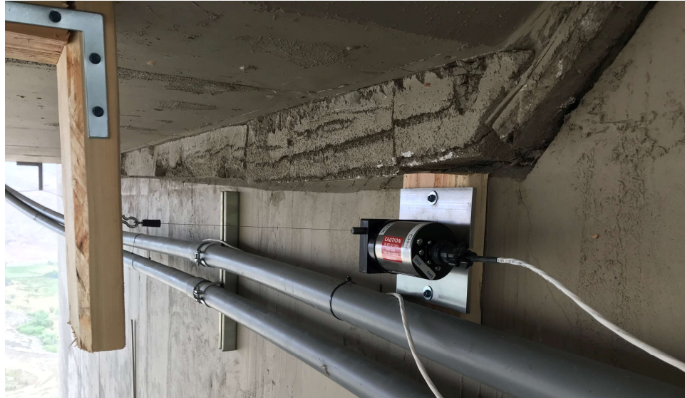
Figure 4.12: Potentiometer located at west edge of Abutment 1 of northbound structure
