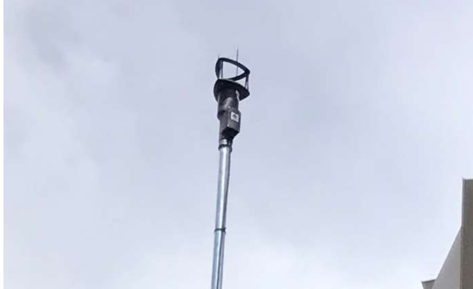
Figure 4.16: R.M. Young 86000 ultrasonic anemometer installed at utility shed
